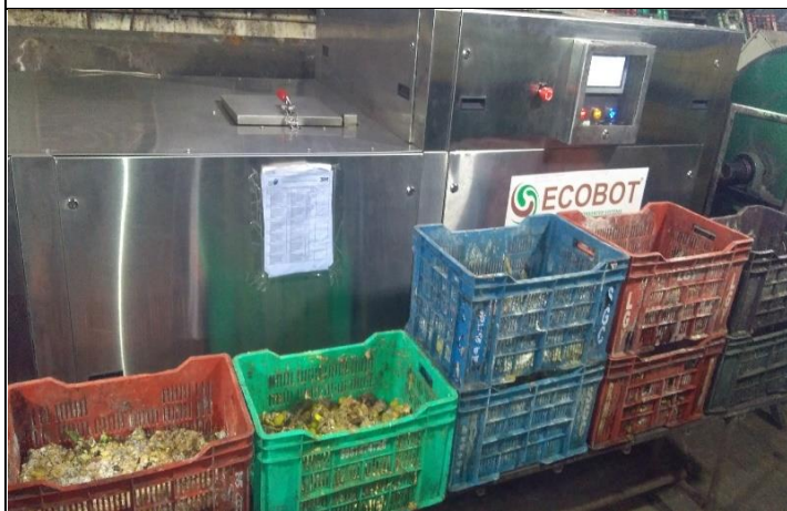
7. Installation of organic waste composting machine With capacity to compost 500 kg of food waste daily.
